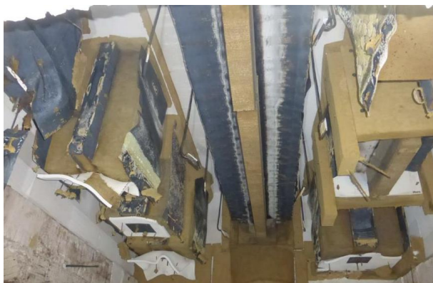
a) Disbonding of the fire-exposed steel sheets of sandwich panels
